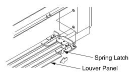
Figure 36 - Removing Louver Panel
